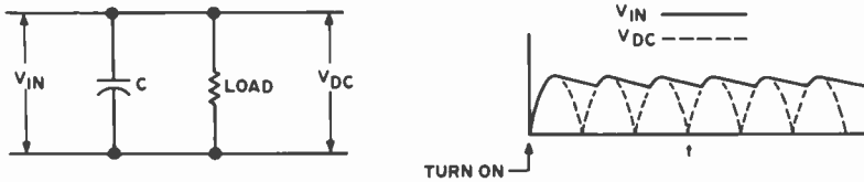
Figure 3: Using a Capacitor for Filtering. The capacitor charges up whenever a voltage is applied, and the load resistance tends to discharge the capacitor. The net result is a tendency for the voltage to remain approximately constant with ripple left over from the rectification.
